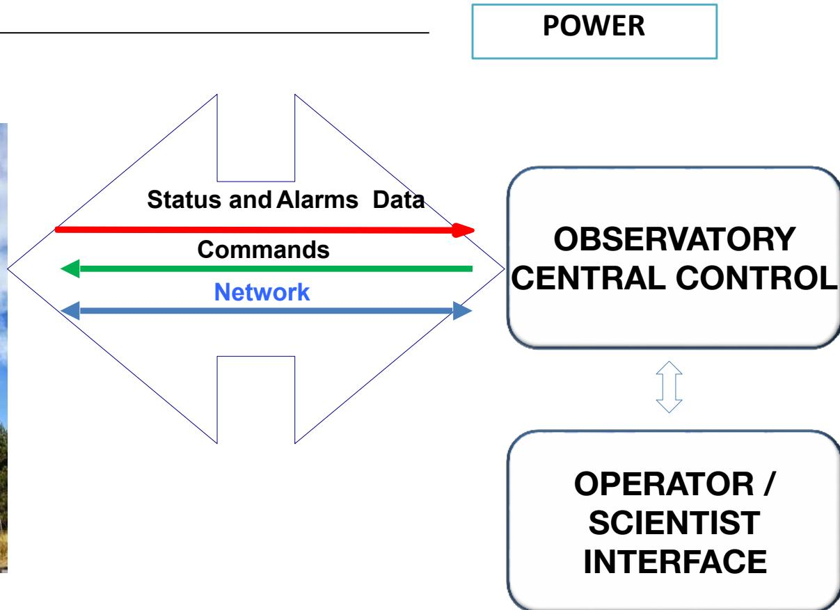
The ASTRI SST-2M is a stand-alone intelligent active machine programmed to receive commands, acquire and transmit scientific/engineering data, detect, signal and, where possible, recover from errors.
