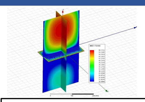
to provide, with some of the X-IFU filters proper Radio Frequency shielding in the frequency range of the satellite telemetry.
