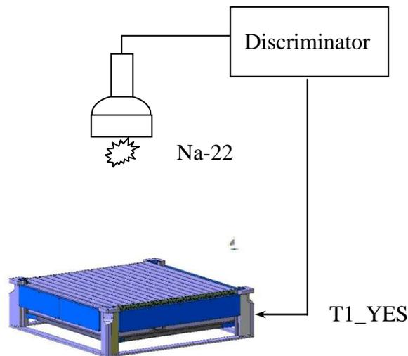
**Figure 6-2-1 GRID acquisition scenario. A Na-22 source will be placed above MCAL and will be monitored with a detector that will generate the T1\_YES signals needed in the GRID**
