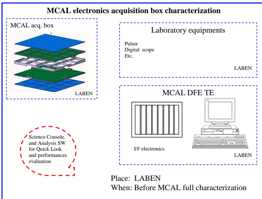
Figure 5-4-1 MCAL acquisition box characterization scenario. Blue contour indicates a LABEN responsibility, red contour a IASF-BO responsibility.
