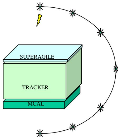
**Figure 7.3.1: Source positioning pattern of the flood measures to be performed with uncollimated sources at different angles  $\phi$ . AC is not shown for clarity.**
