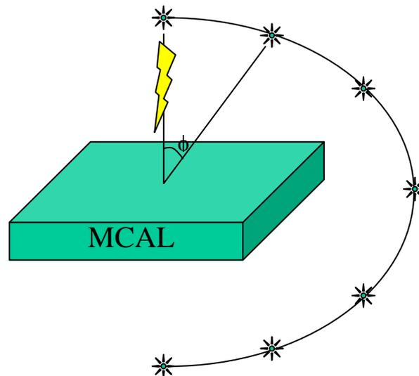
**Figure 6.3.1: Source positioning pattern of the flood measures to be performed with uncollimated sources.**
