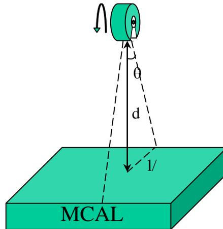
**Figure 6.4.1: Possible Burst simulator showing the rotating chopper with the source inside.**
