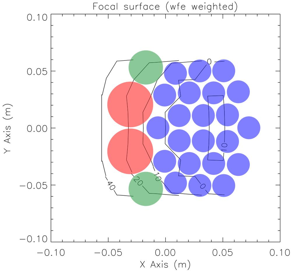
Figure 14: A possible focal plane with 2 feed horns at 35 GHz (in red), 2 feed horns at 45 GHz (in green), and 22 feed horns at 94 GHz (in blue).
