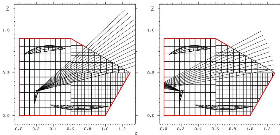
Figure 8: *Left side*: contribution due to diffracted rays from the lateral panel (Dl7). *Right side*: contribution due to rays reflected by the panel reflector\_d (Rd).
