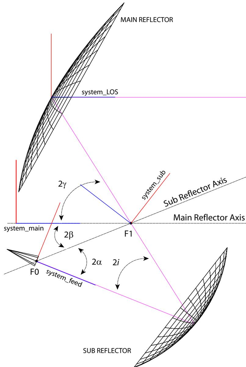
Figure 1: Telescope geometry.
