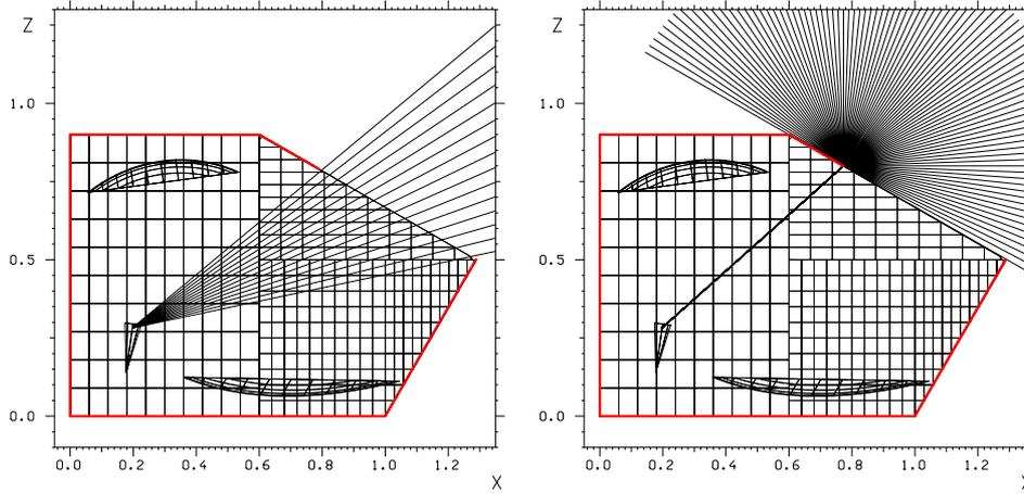
Figure 6: *Left side*: direct contribution from the feed. *Right side*: contribution due to diffracted rays from the front-top panel (Dft).
