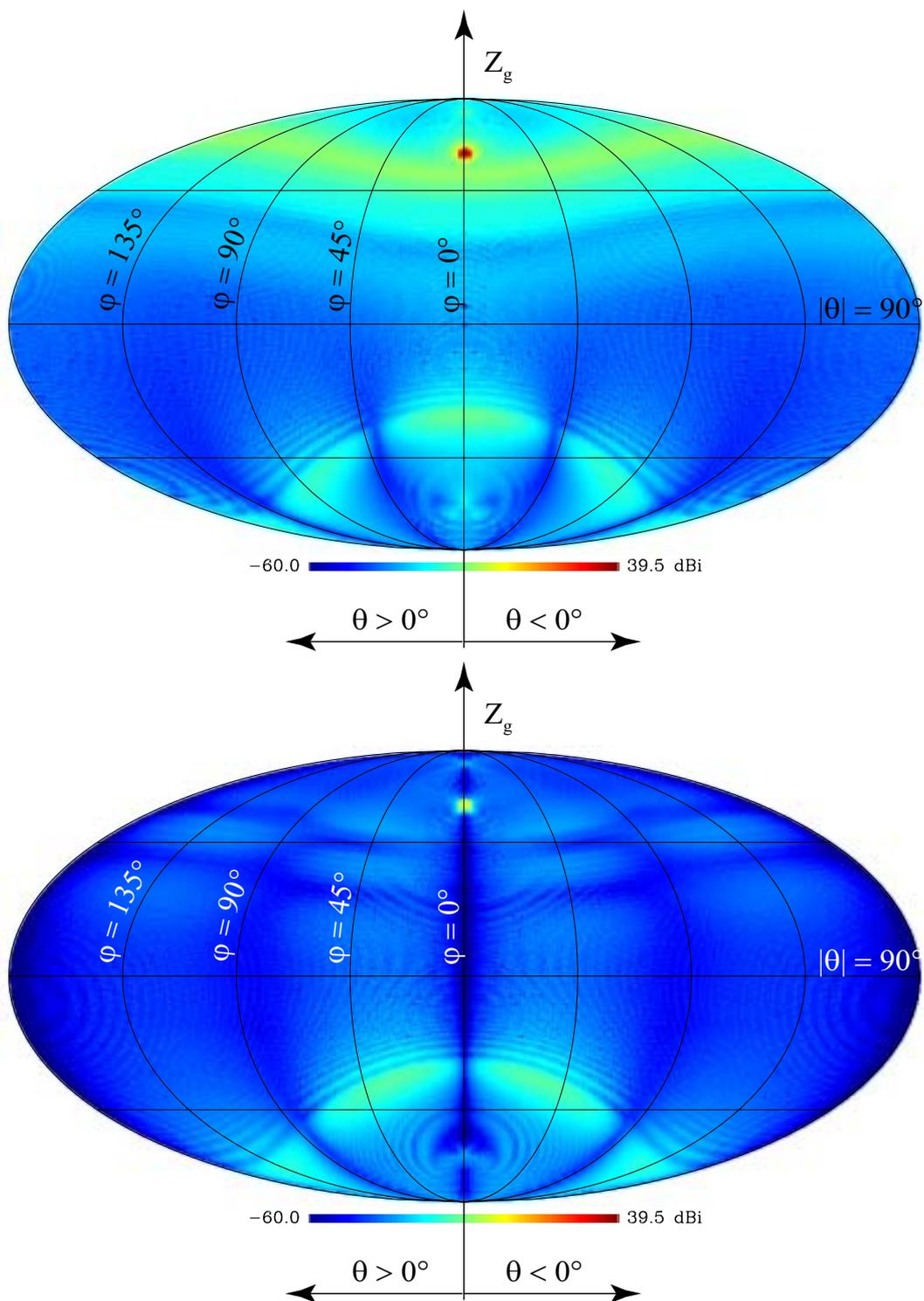
Figure 4: Co- and cross-polar component of the beam computed with PO/PTD, without shields.
