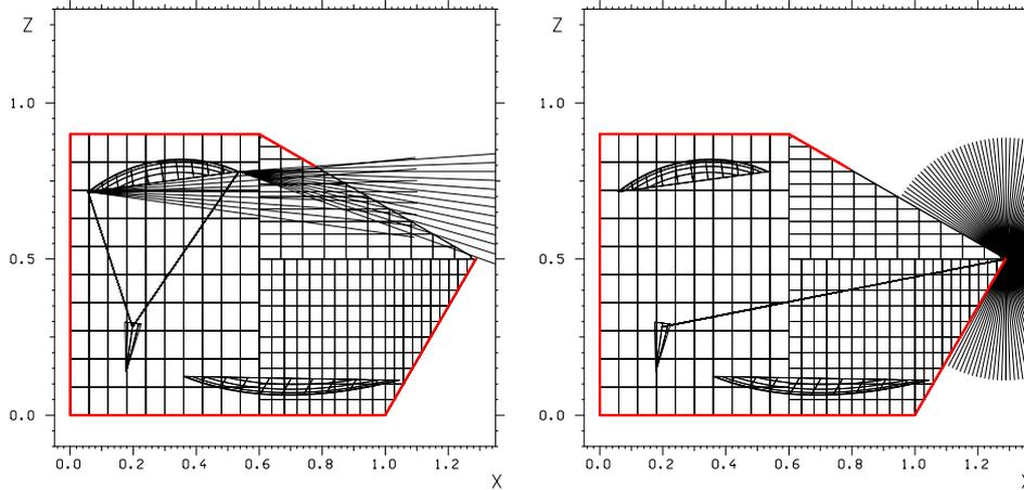
Figure 7: *Left side*: contribution due to diffracted rays from the sub reflector (Ds). *Right side*: contribution due to diffracted rays from the front-bottom panel (Dfb).
