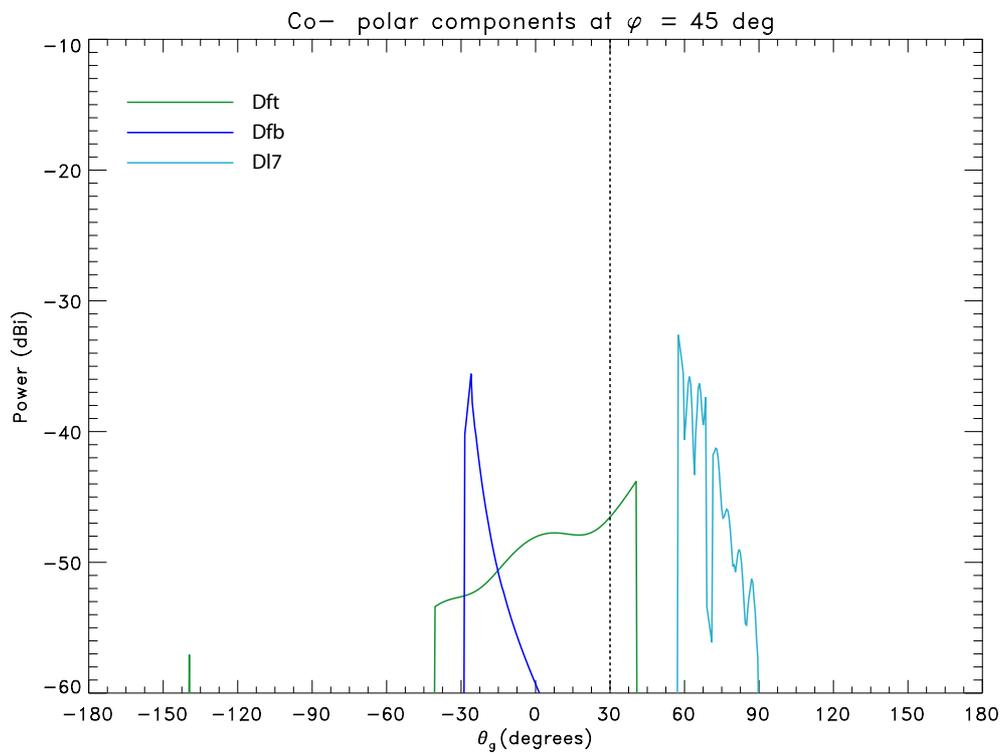
Figure 10: Relevant MrGTD contributions in the plane  $\phi = 45^\circ$ .
