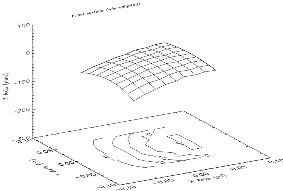
Figure 13: Focal surface that minimize the weighted wave front error.
