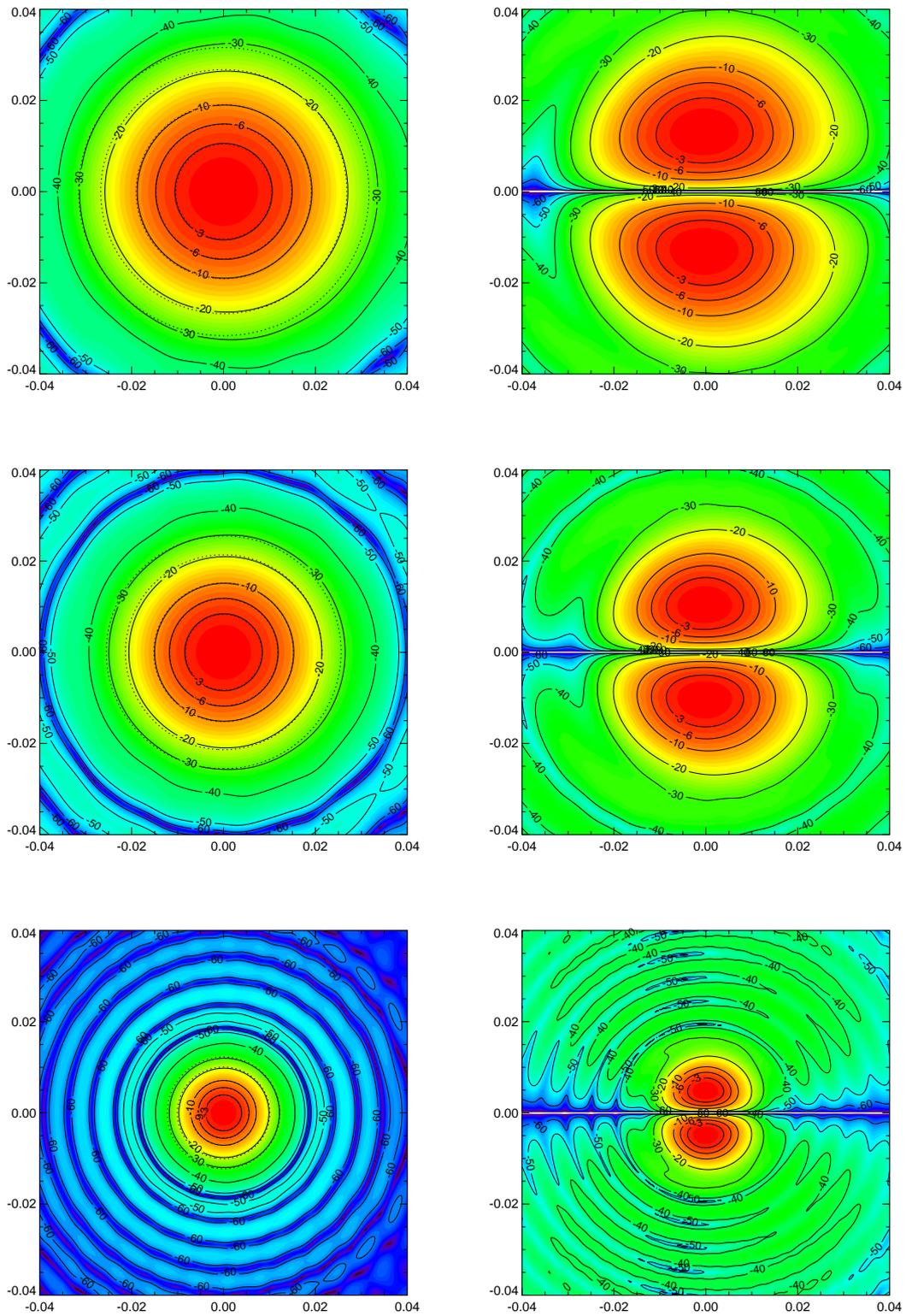
Figure 3: Co- and cross- polar components of the main beams at 35, 44, and 94 GHz.
