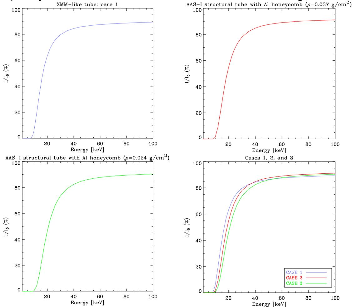
**Figure 2:** Absorber transparency, expressed as the ratio  $I/I_0$  (in %) between undetected and incident radiation as a function of photon energy, calculated for the shield compositions of Cases 1, 2, 3, described in Section 1:
