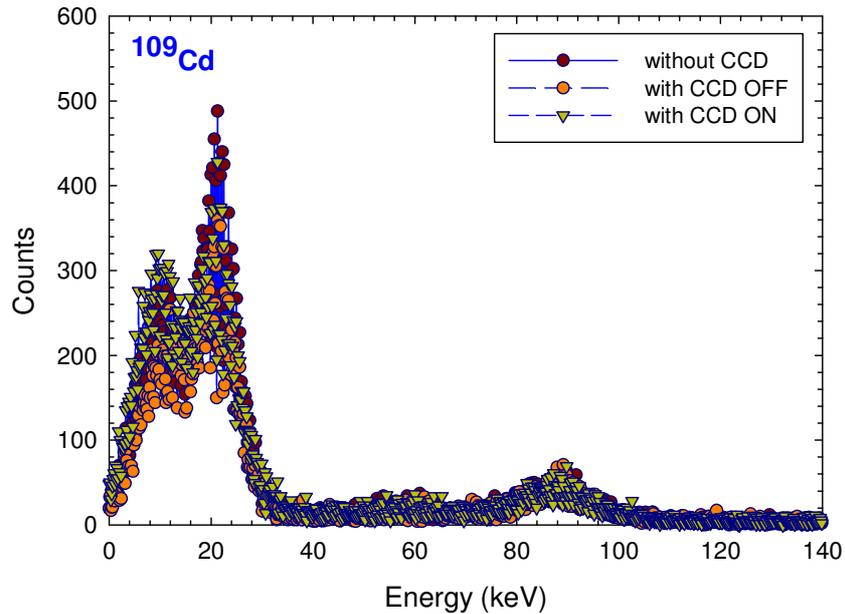
Figure 15. Measurement acquired without CCD in front of the CZT pixel detector; with CCD turned off in front of the CZT array and with CCD switched on using the sources of  $^{55}\text{Fe}$  and  $^{109}\text{Cd}$ . We have reported the sum of the analysed spectra.
