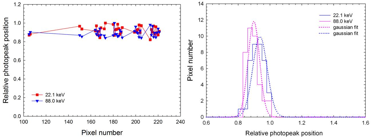
Figure 5. Behaviour of the photopeak centroid of the examined pixels at 22.1 and 88 keV, each value is normalized to the relative maximum (left); histogram of the centroid values (right).
