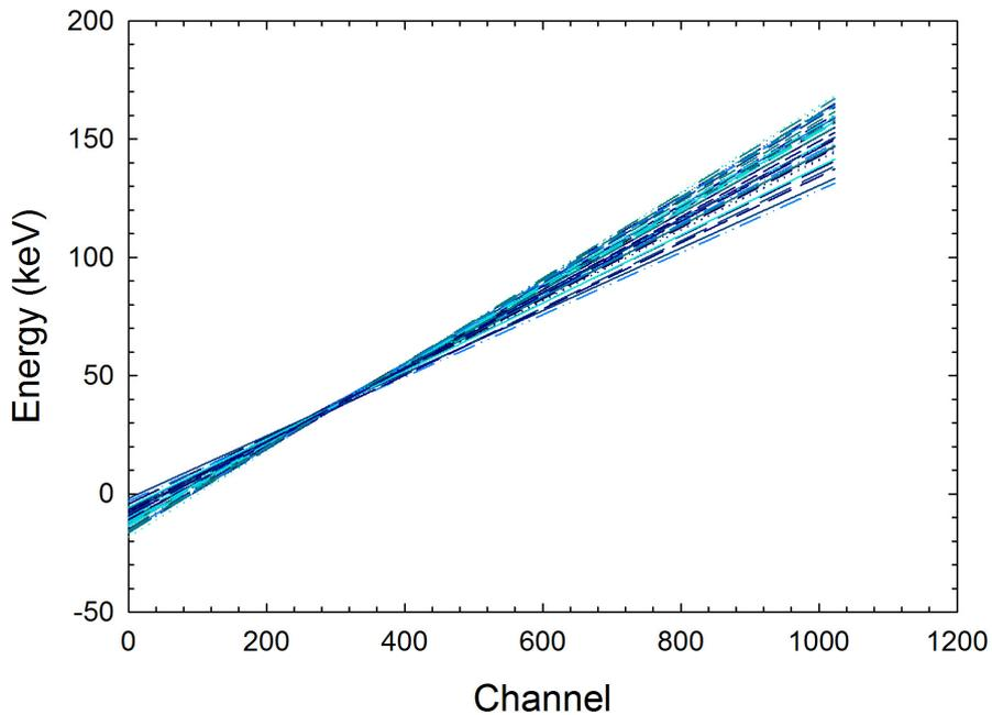
Figure 4. Calibration curves obtained using the centroids at 22.1 and 88 keV. The equalization of the channels was done in another environment at 1% level about six months before, but there was no time to repeat it.
