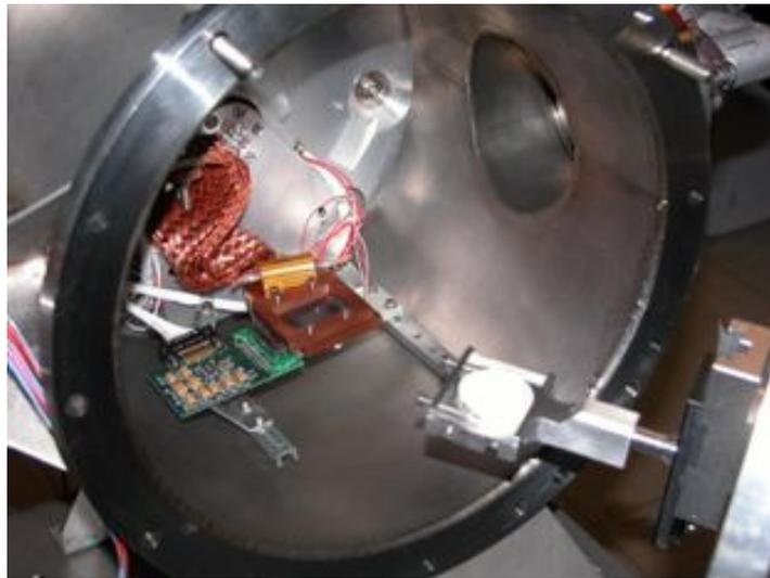
Figure 9. Vacuum chamber containing the CCD.
