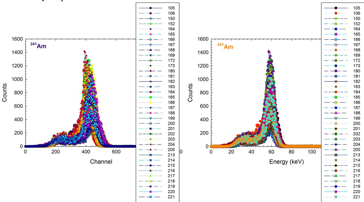
Figure 11. Energy spectra of  $^{241}\text{Am}$  before (left) and after calibration (right).
