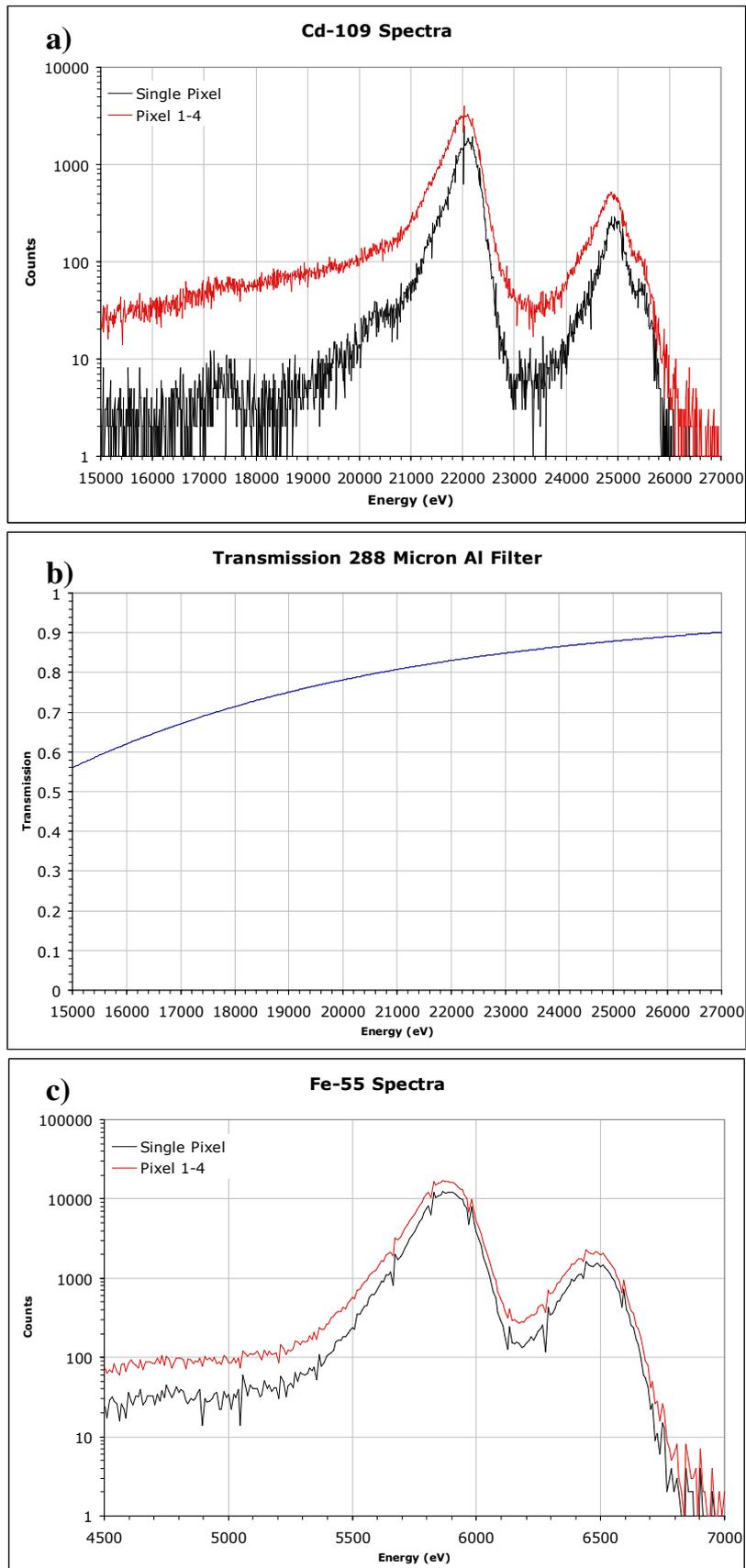
Figure 8. a) Pulse height spectrum recorded with  $^{109}\text{Cd}$  source; b) transmission calculated for the 288 micron Al filter; c) spectrum acquired with  $^{55}\text{Fe}$  without attenuating filter.
