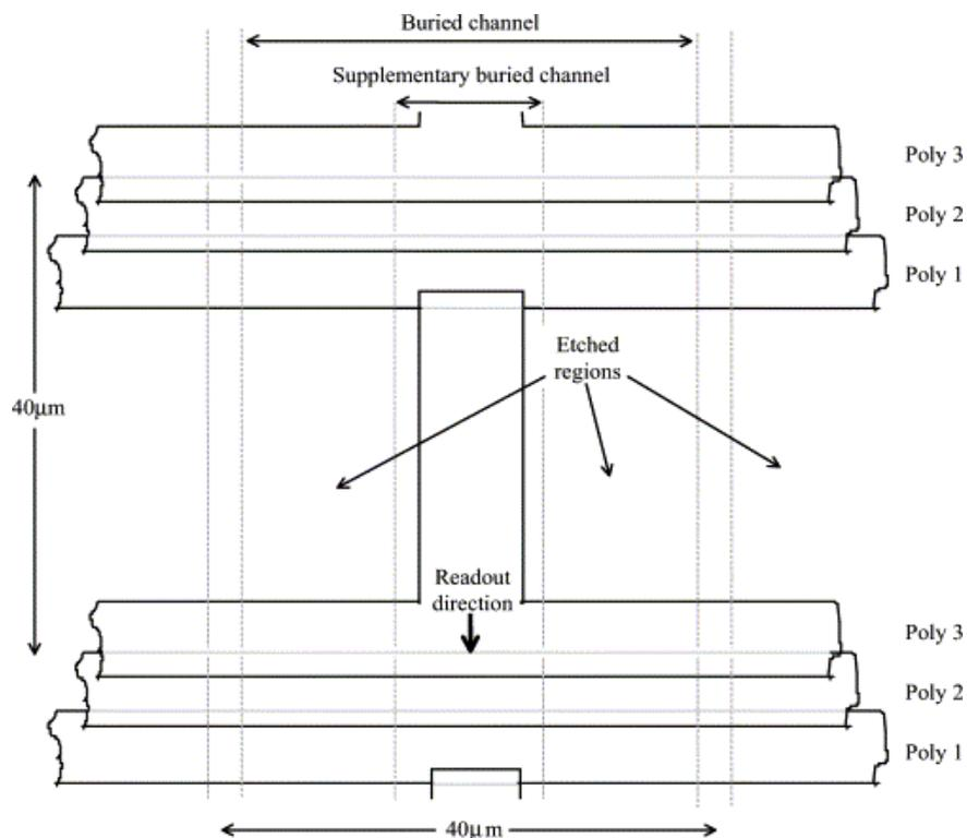
Figure 7. Simplified CCD22 electrode structure.
