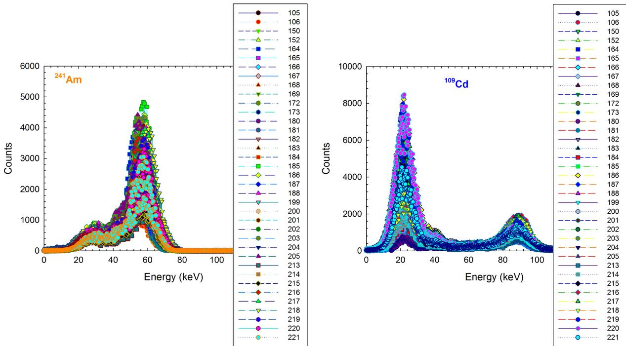
Figure 3. Energy spectra of  $^{241}\text{Am}$  (left) and  $^{109}\text{Cd}$  (right) acquired by illuminating ~40 pixels.
