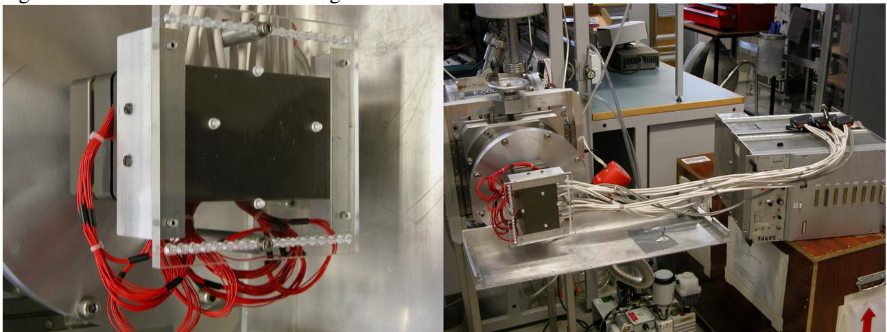
Figure 10. The pixel detector on the left; overall view of the used system on the right.
