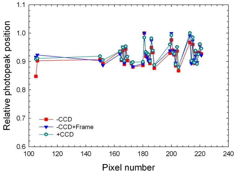
Figure 12. Behaviour of the photopeak centroid at 59.54 keV.
