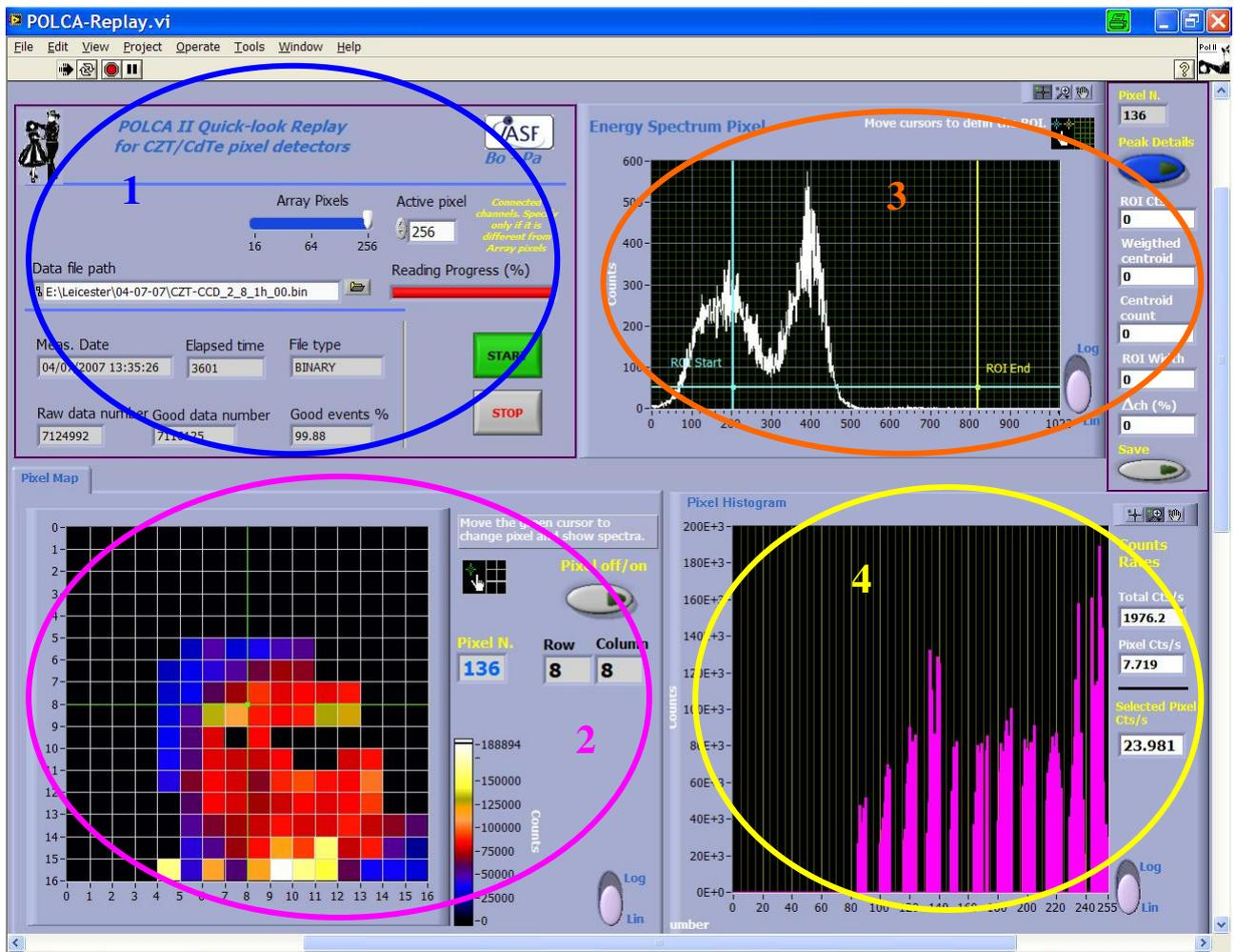
Figure 13. Main control panel of the software realized in LabVIEW to read the stored measurements.
