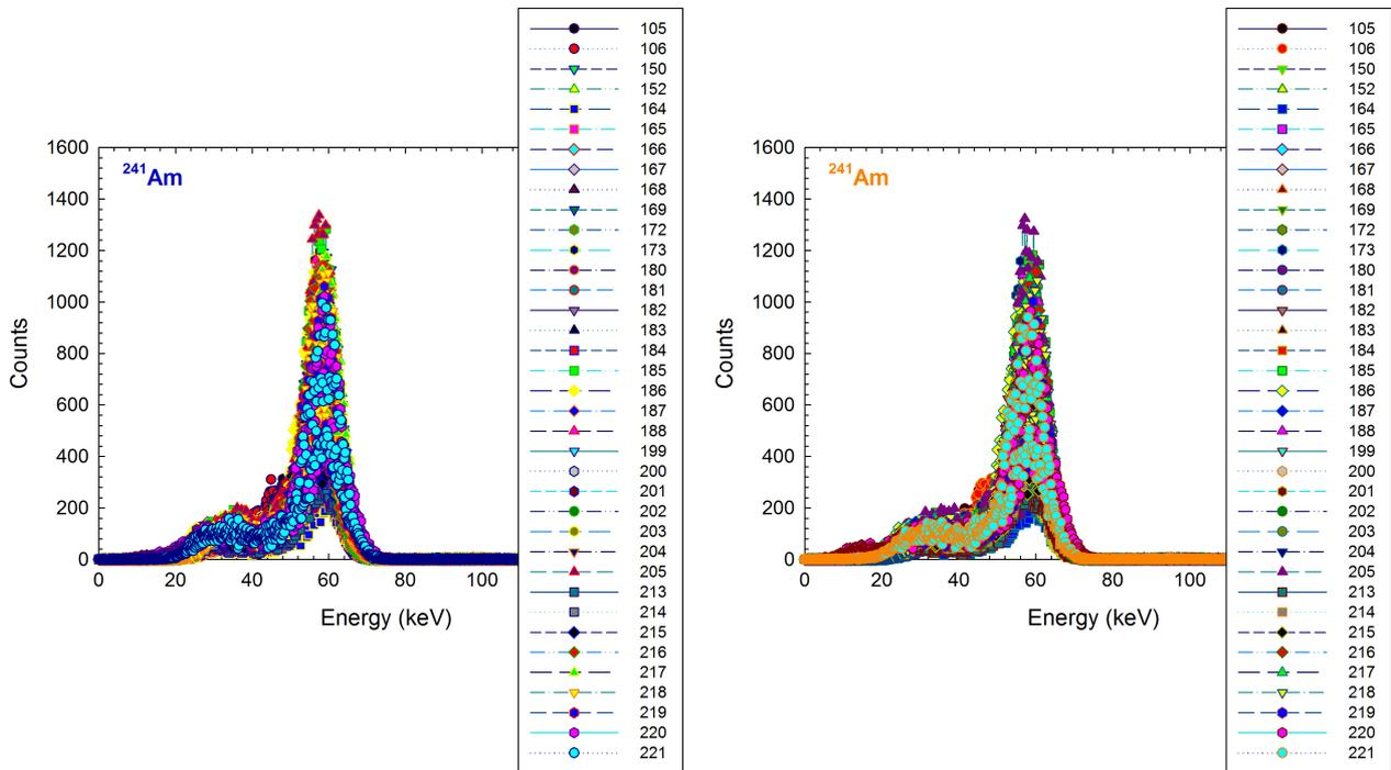
Figure 14. Measurement recorded without CCD in front of the CZT pixel detector (left); with CCD turned on in front of the CZT array (right) by irradiating with the  $^{241}\text{Am}$  source .
