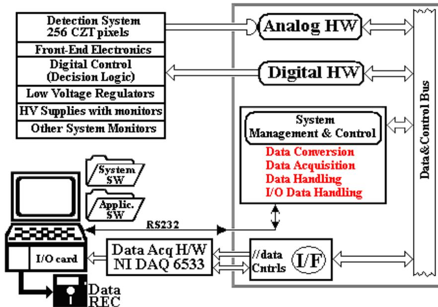
Figure 2. The functional scheme of the detection system: (left top box) the CZT pixel detector with the Analogue front-end electronics; (right box) the multiparametric data processing.
