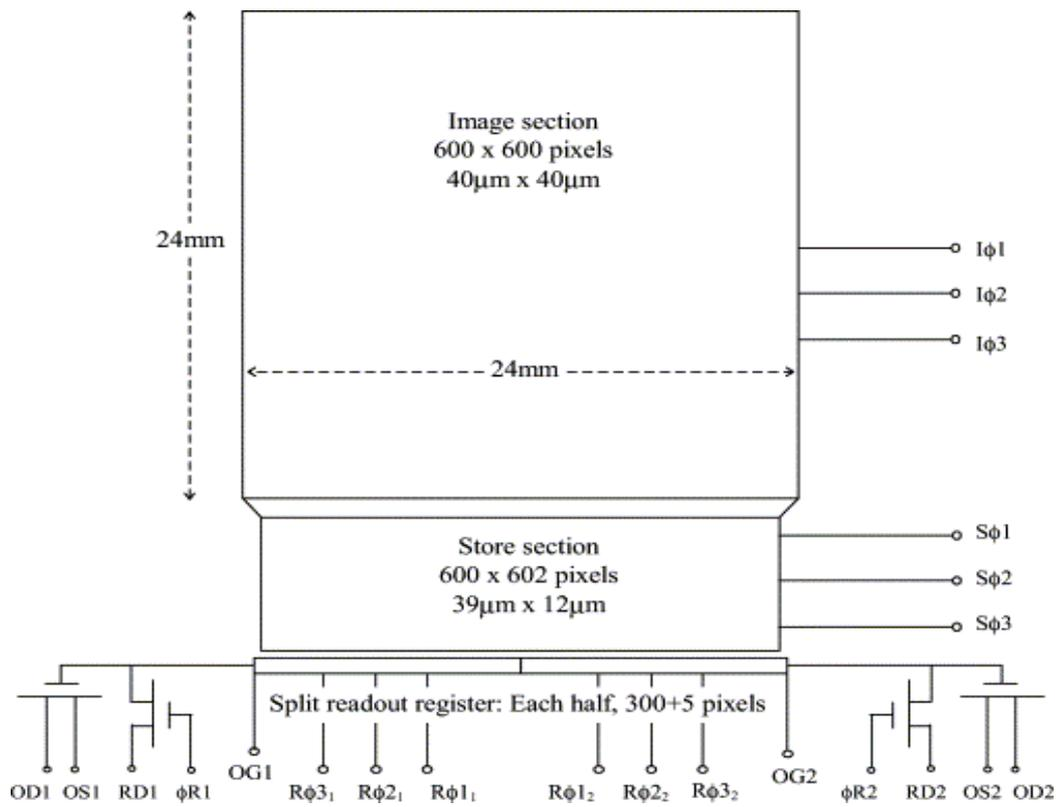
Figure 6. CCD22 simplified schematic.
