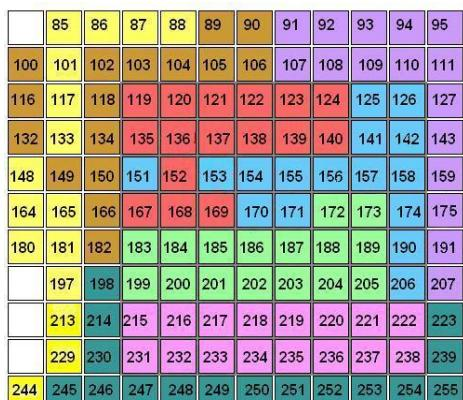
**Figure 7.** The ASIC chip/pixel association for the POLCA II detector.
