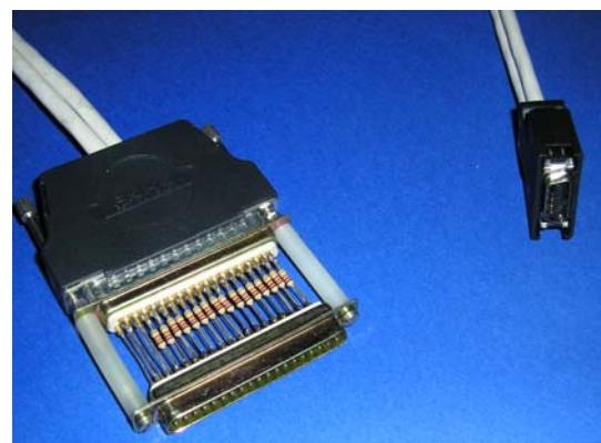
**Figure 2.** The new data cables and connectors (left); the new 12 kΩ resistor set at the end (TAKES) of the data cable (right).
