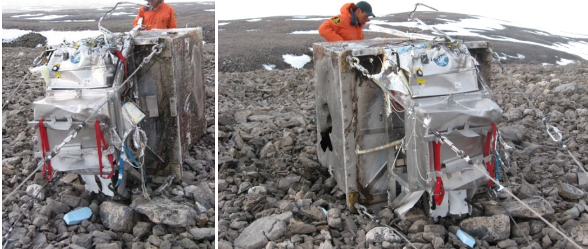
Figure 1. The SORA gondola after the landing on the 15 th July 2009 (9h:24':13''). The crashed envelope of the Telemetry box (with the light blue sticker on) containing the BIT unit is visible on the top side.
