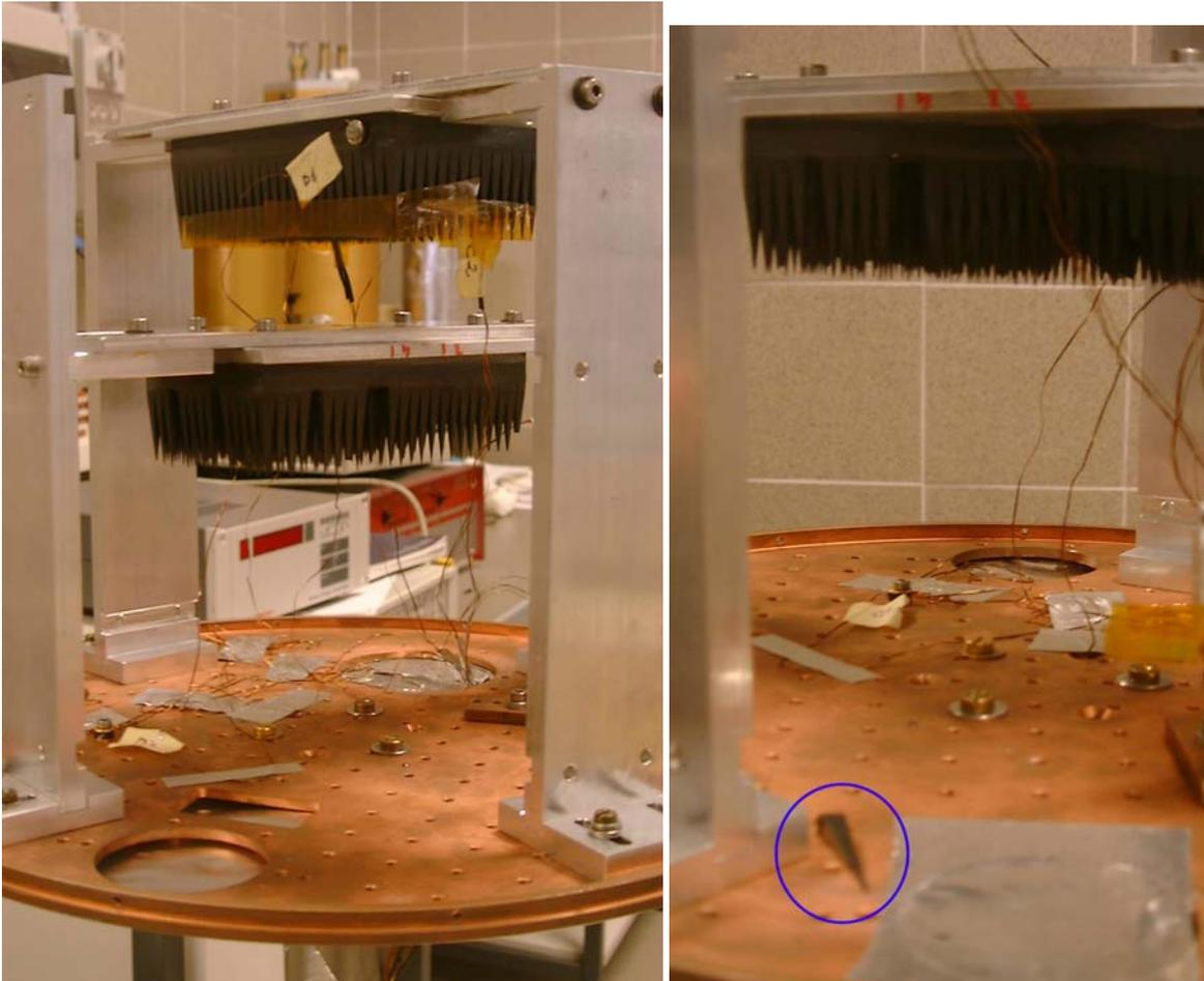
Figure 27 Global view of the samples mounting after opening the CF. In the right picture, the broken pyramid is visible.
