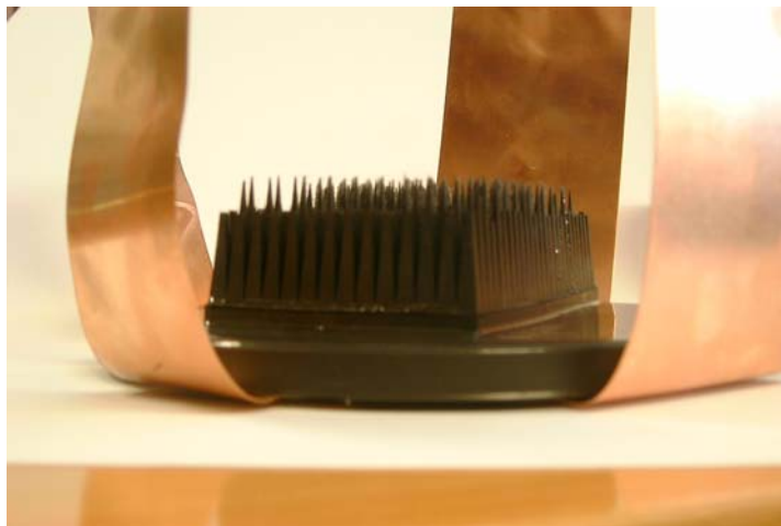
Fig. 2 Global view of the sample. The pyramid panel is visible together with copper thermal straps.
