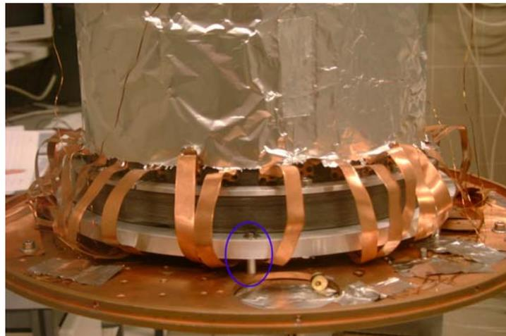
Fig. 1 Sky Load mounted on the facility cold flange. Lateral wall copper slabs links to the Aluminum base and a stainless steel washer (blue circle) are visible.
