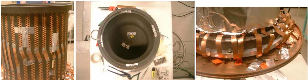
Fig. 3 Sensors locations. Sensors A and C3 are displayed in the left panel, sensors B, D1, D2, D3, D4 in central panel and sensors C1, C4 in the right panel.
