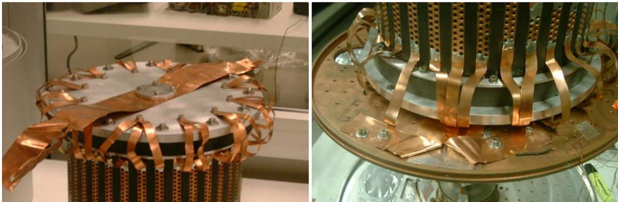
Fig. 2 A wide copper slab is attached to the Aluminum base (left figure) and then fixed to the facility cold flange (right figure).
