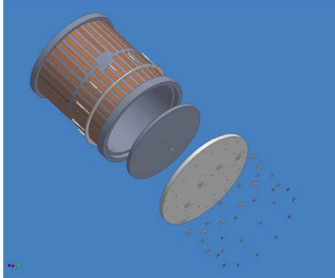
Fig. 4 Exploded view of the load cylinder. The Eccosorb base is hold by the Al base screwed to an Eccosorb step on the bottom of the cylinder wall with the help of disc springs.
