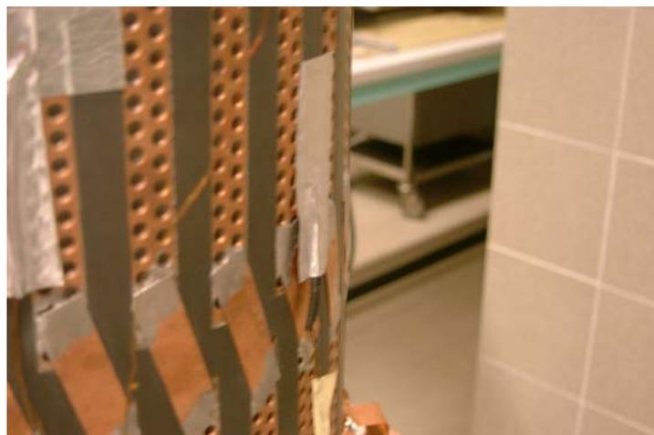
Fig. 12 Aluminum tape on the lateral wall sensors was found slightly detached.
