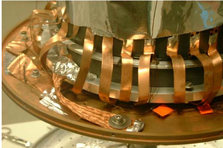
Fig. 9 Detail of one of the three thermal straps added in the third cycle
