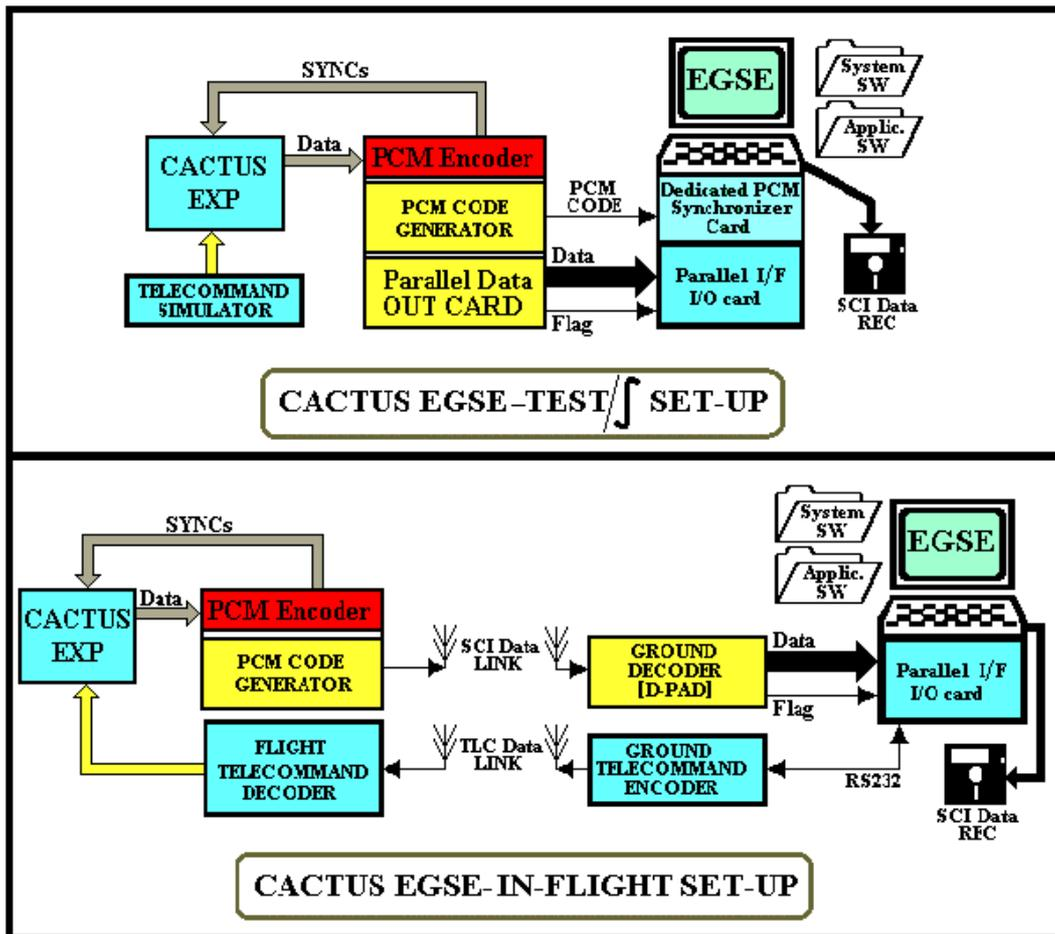
Figure 5. Two possible and equivalent configuration for the Cactus experiment EGSE.
