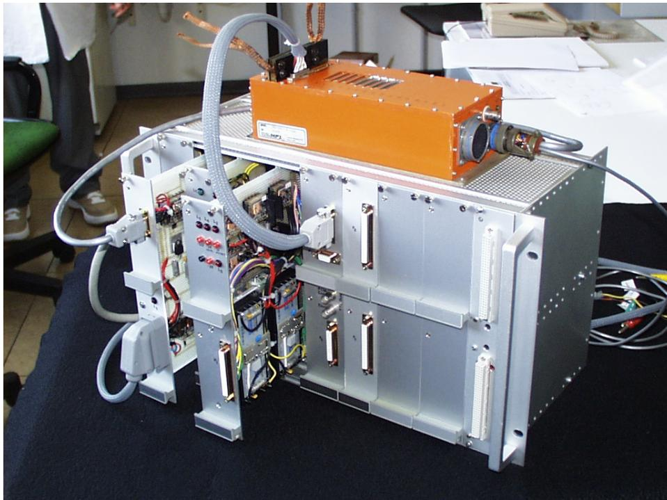
**Photo 4.** Another view of the Cactus Service Electronics with the PCM Encoder (Metraplex 760) box above.
