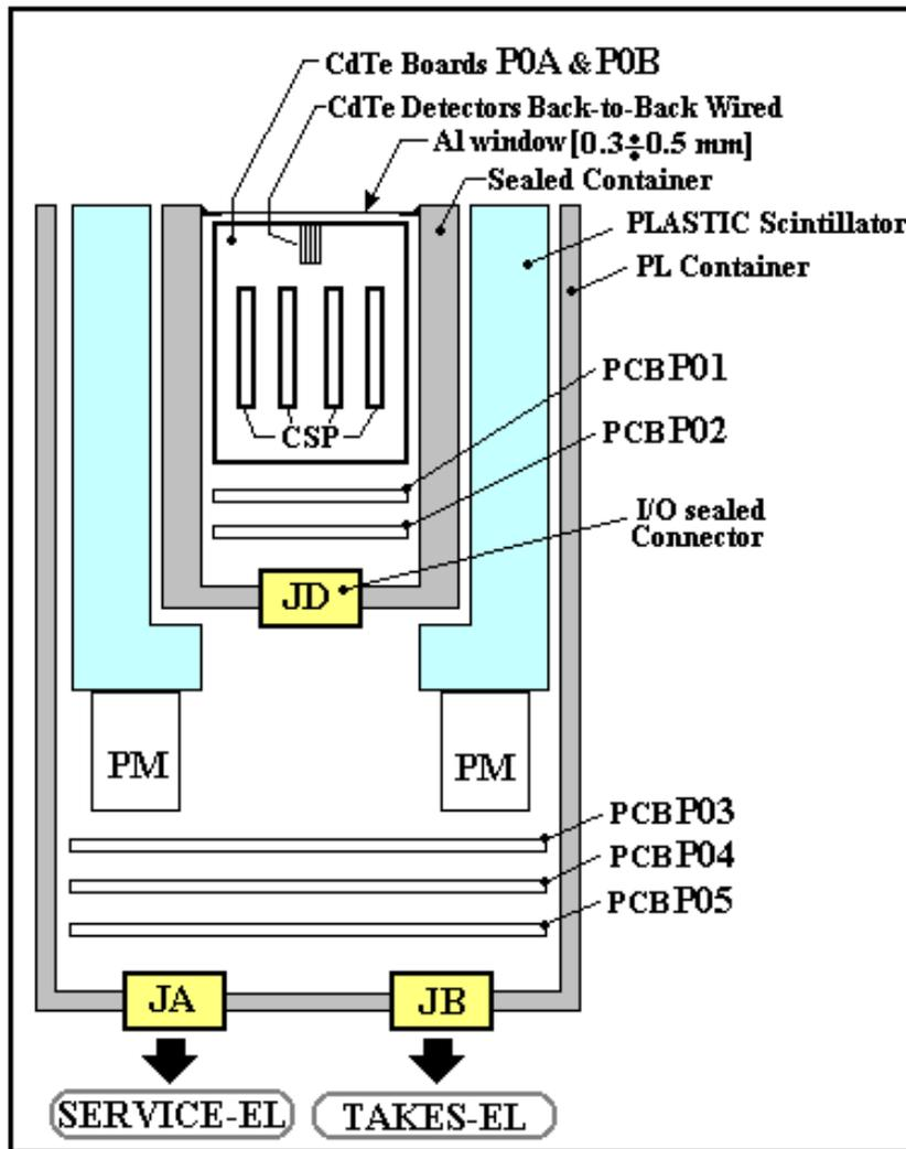
**Figure 2.** The scheme of the Cactus detector
