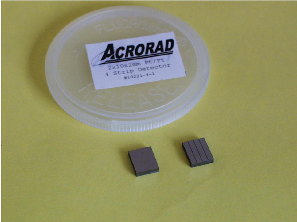
**Photo 1.** The Cactus CdTe detection units from Acrorad (Japan): the cathode surface (left), the multistrip anode side (right).
