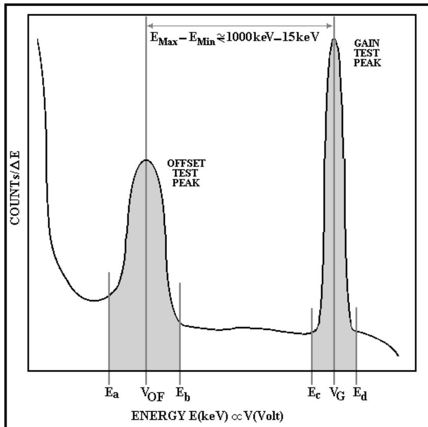
**Figure 4.** Self Test and calibration procedure on FE electronics
