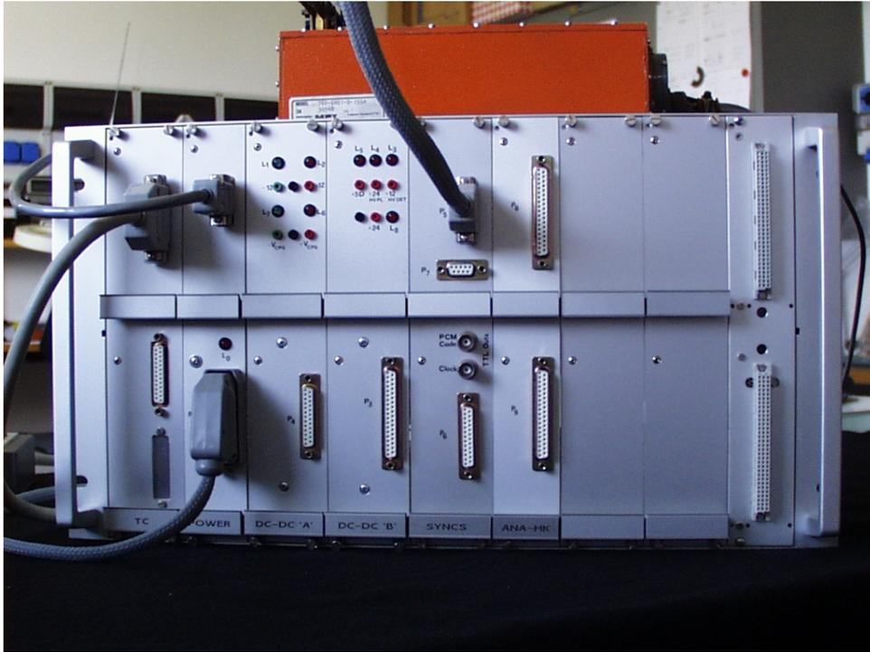
**Photo 3.** A front view of the Cactus Service Electronics. The modules are from left to right: the Telecommand unit, the Power, DC-DC converters for CSP and electronics module, the DC-DC converters for CdTe detectors and Plastic HV and for digital electronics bias module, Synchronism unit and Analog House keeping module.
