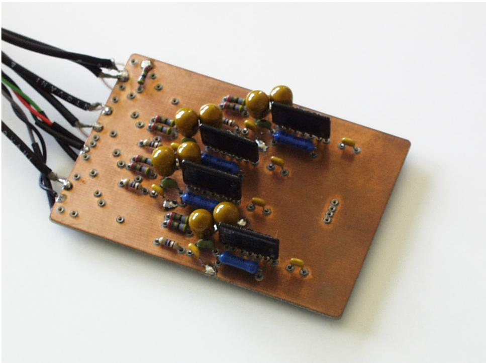
**Photo 2.** The front-end readout electronics board with the charge sensitive preamplifier (black elements) Clear Pulse CS-515 and the analog filters for HV and low bias.
