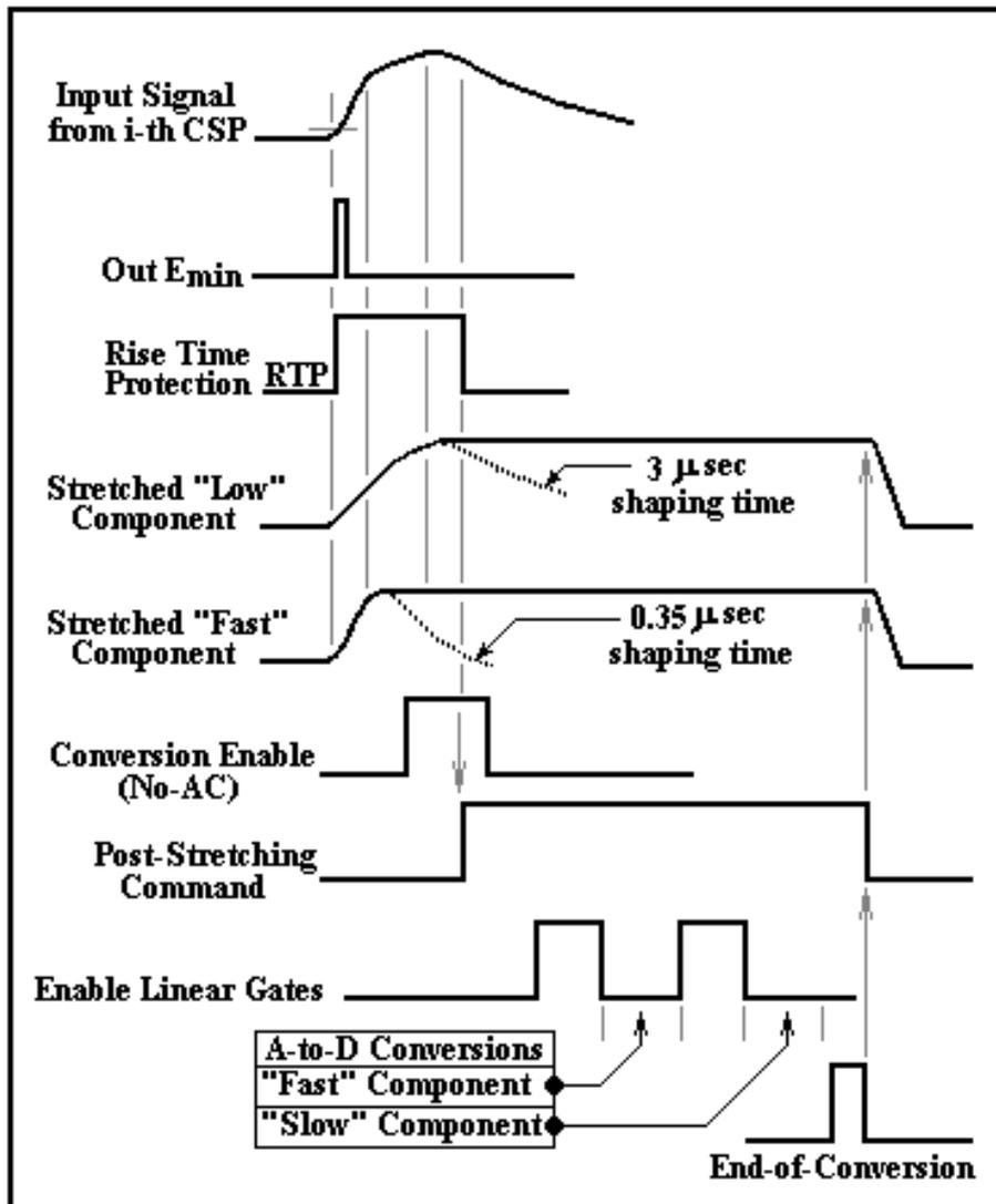
**Figure 3.** Typical waveform diagram with no veto signals.
