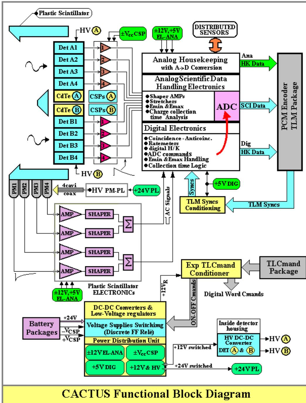
**Figure 1.** The Cactus functional block diagram. All the experiment subsystems with their functional links are shown.
