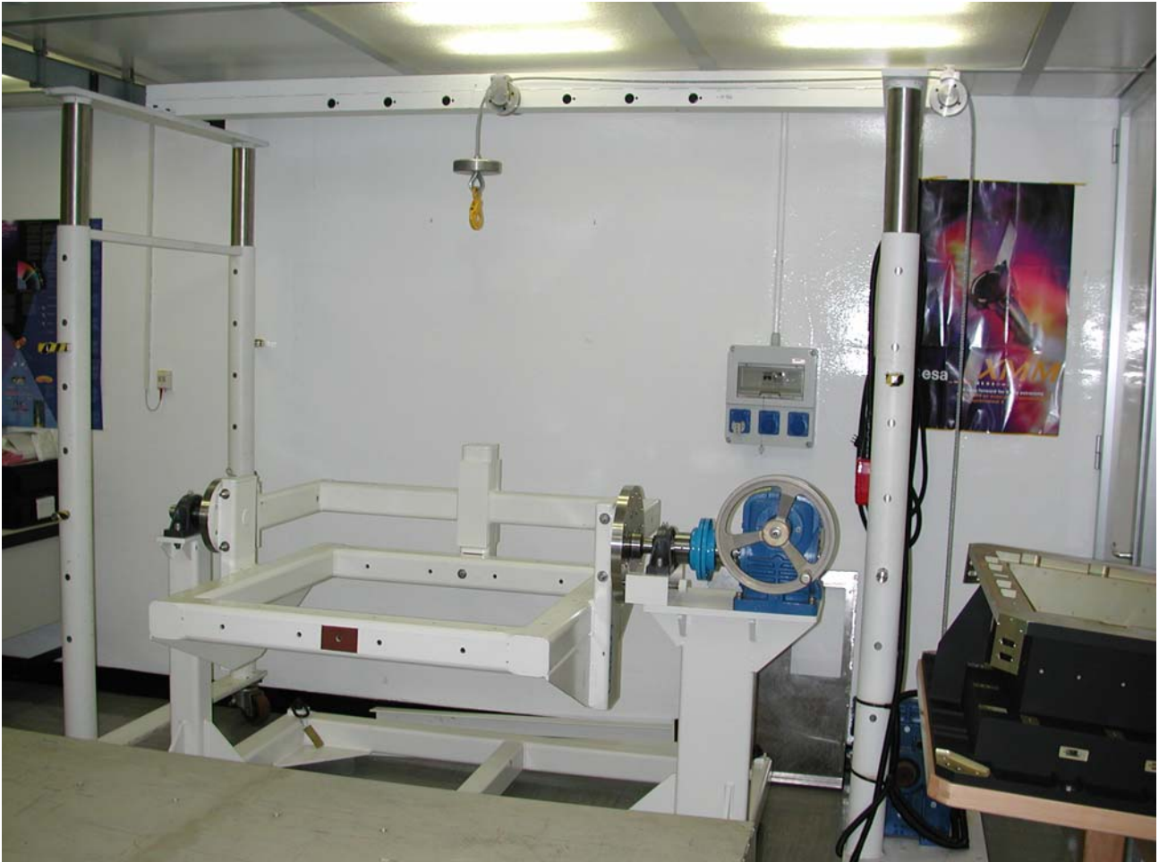
Figure 5-1 LABEN Travelling Crane with the IBIS Rotating Table
