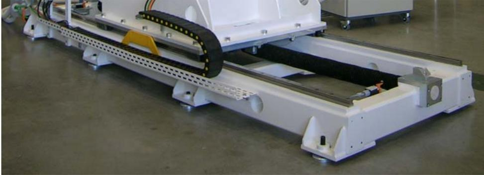
Figure 7-1 Levelling screws
