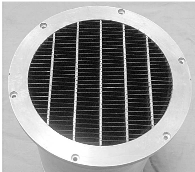
Figure 1: Realization of the first collimator solution above the High Energy instrument aboard HXMT.
